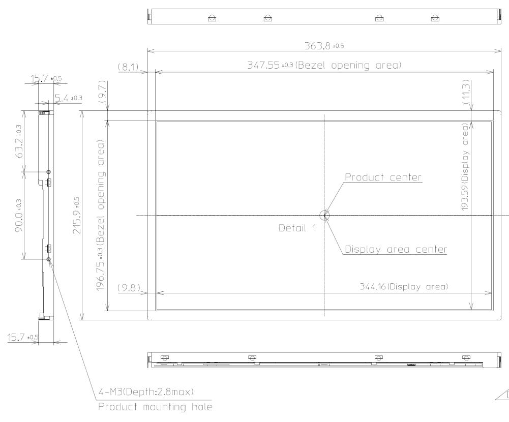
Note1: The values in parentheses are for reference. Note2: The torque for product mounting screws must never exceed 0.34N·m. And the length of product mounting screws must be  $\leq$  2.8mm.
