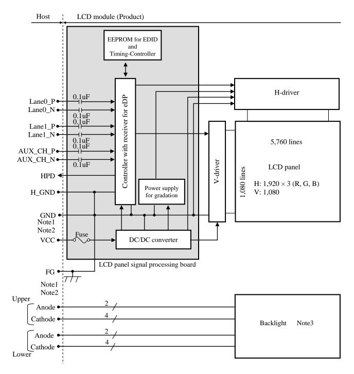
Note1: Relations between H\_GND (High Speed Ground), GND (Signal ground) and FG (Frame ground) in the LCD module are as follows.
