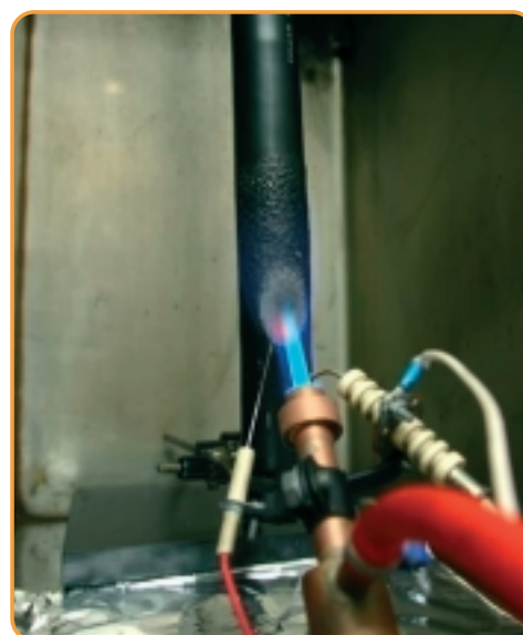
Test on flammability of single cables.
