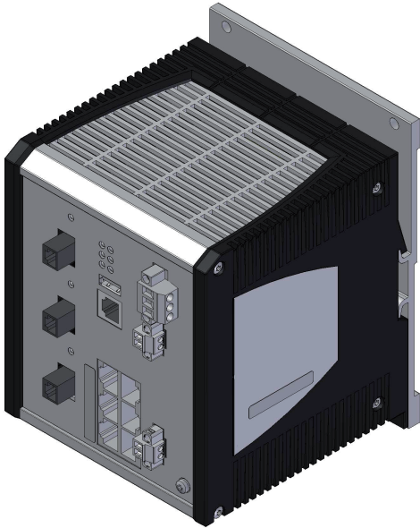
Figure 20: Mounting the RS22/RS32 devices on the wall
