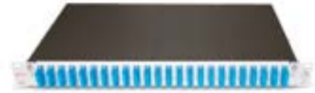
Splice box OV-S, 19"/1U, extractable, Example with 24 SCD adapters / 48 pigtails
