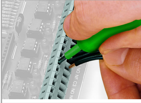
Inserting a conductor via 3.5 mm screwdriver.
