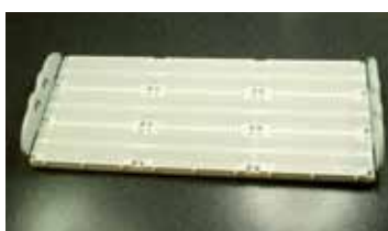
Stackable, interchangeable, removable 4995 point testboard
