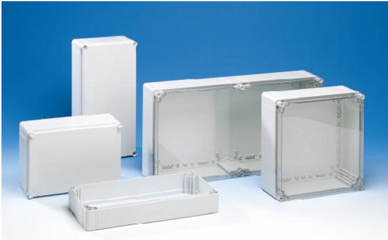
A durable and versatile enclosure has been the main concept for the construction of the CUBO O range. The enclosures are made of polycarbonate and ABS. Extension frames and alternatives for fastening of covers give a variety of possibilities. Adjustable elevators in the base corners allow mounting of plates and panels at any height. Standard colour is grey RAL 7035. The covers are grey or transparent. Degree of protection IP 66/67.
