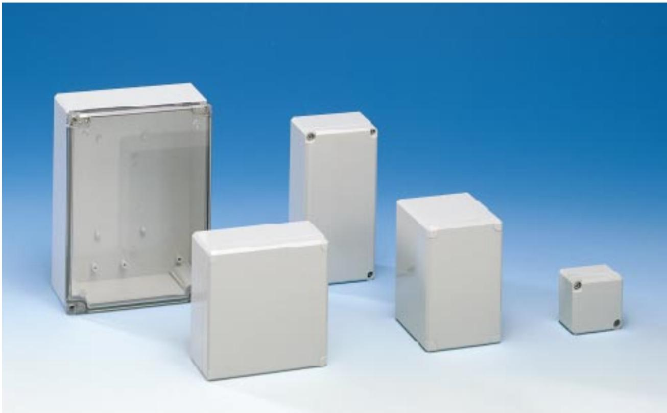
The CUBO D enclosure range is designed for housing of sensitive electronic, electric and pneumatic components and for use as terminal box. Special features are fastening pods inside the cover, slots for circuit boards in the base and cover plugs for the cover screws.
