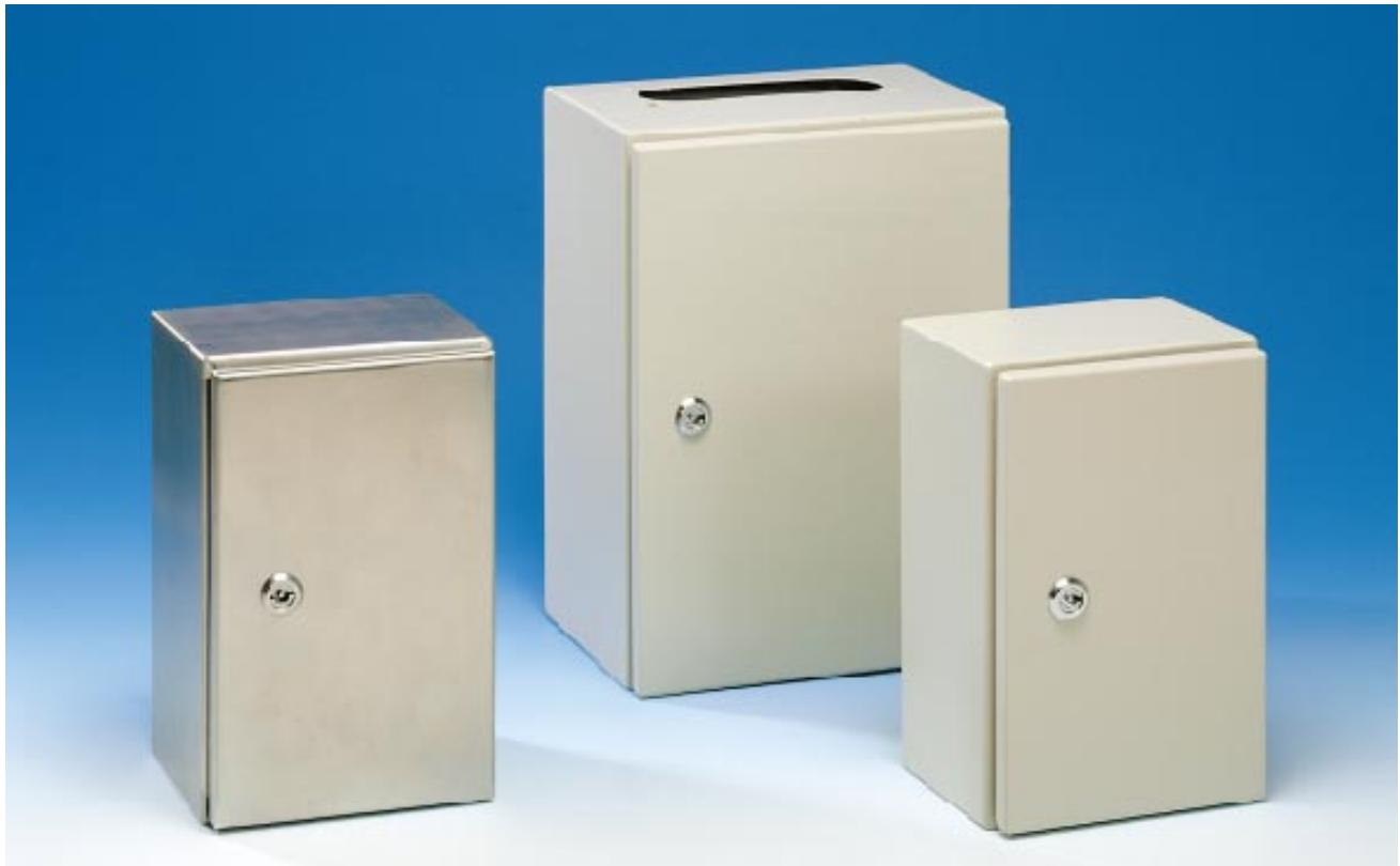
The metal E-range of enclosures (EFE, ESSP and EAS) is made either of painted sheet steel or unpainted stainless or acidproof steel. Corrosion resistance is achieved by a zink-phosphate surface treatment and relief structured polyester powder paint. Mounting plates, cover plates for flange openings and key are included in the package. The acidproof and stainless steel enclosures have no flange openings.
