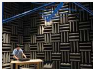
Acoustic radio wave anechoic chamber
