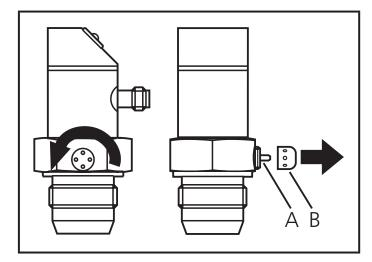
The vent (A) should only be cleaned by skilled personnel and with utmost care. Possible medium residues must not be compressed and pressed into the vent. This could clog the filter system and reduce the measuring accuracy of the sensor.
