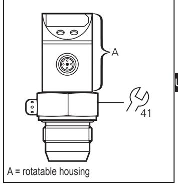
The unit is adaptable for various G 1 process fittings. G 1 process adapters to be ordered separately as accessories.
