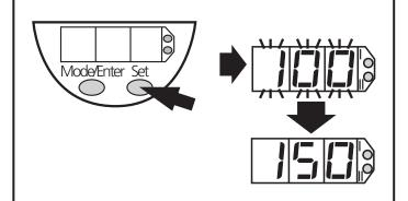
The numerical values are incremented continuously. If the value is to be reduced: Let the display move to the maximum setting value. Then the cycle starts again at the minimum setting value.
