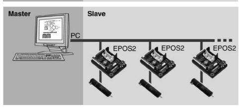
EPOS2 is a modular constructed digital positioning controller. It is suitable for DC and EC motors with incremental encoder with a power range from 1 to 700 watts continuous power. A number of operating modes provides flexible application in a wide range of drive systems in automation technology and mechatronics.
