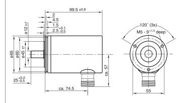
Model No. 66 with clamping flange and shaft with flat
