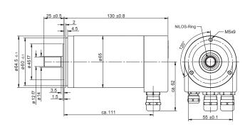
Model No. 66 with clamping flange and shaft with flat
