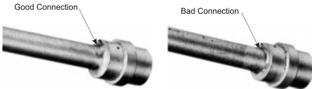
Figure 2-4. Examples of Good and Bad Solder Connections
