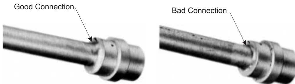
Figure 1-3. Examples of Good and Bad Solder Connections
