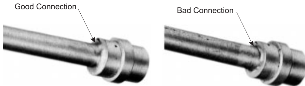
Figure 3-4. Examples of Good and Bad Solder Connections
