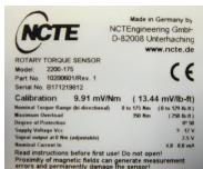
V<sub>out(max)</sub> and V<sub>out(min)</sub> are defined with the slope of the sensor. i.e. the output voltage could be between 0.5 V and 4.5 V. The actual signal output range depends however on the calibration value.
