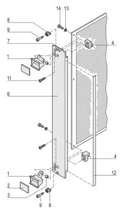
Plug-in units with trapeziform extractor handle, type 1 – front panel, U-profile, shielded
