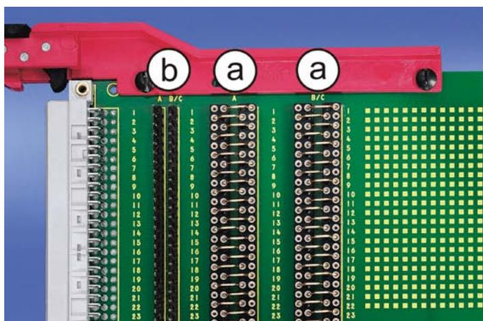
a: Measuring field for current and voltage measurement
