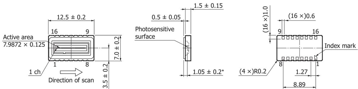
\* Distance from the outer of the window to the photosensitive surface
