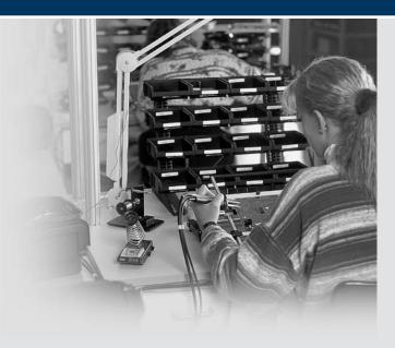
raacostat naturally fulfils the EN 61340-5-1 standard and all other international requirements. Surface resistance: 10 (4)-10 (9) Ω.
