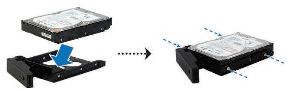
• For 2.5" Hard Disk: Place the hard disk in the blue area (shown below) of the hard drive tray, turn the tray upside down, and then tighten the screws to secure the hard disk.
