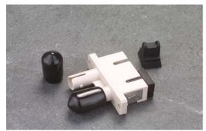
An optical fibre adapter or uniter is used to mate two connectors together, usually mounted in a distribution panel or wall box. In most cases it is the critical part of the system that aligns the ferrule part of the connectors keeping the fibres in perfect alignment.
