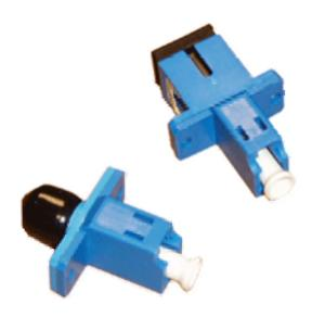
An optical fibre adapter or uniter is used to mate two connectors together, usually mounted in a distribution panel or wall box. In most cases it is the critical part of the system that aligns the ferrule part of the connectors keeping the fibres in perfect alignment.
