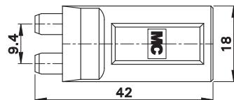
Two-pole test adapter, made of brass with Ø 4 mm rigid sockets at rear for connecting test instrument leads or for feed-ins. Possible uses include measuring the current consumption of connected equipment or measurement of leakage currents in automobile electrical systems without the need to disconnect a wire in an inaccessible place. The adapter is simply inserted in place of the fuse.
