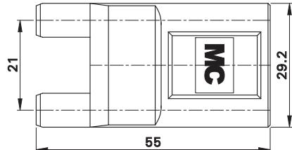
Two-pole test adapter, made of brass with Ø 4 mm rigid sockets at rear for connecting test instrument leads or for feed-ins. Possible uses include measuring the current consumption of connected equipment or measurement of leakage currents in automobile electrical systems without the need to disconnect a wire in an inaccessible place. The adapter is simply inserted in place of the fuse.
