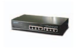
For cost saving and flexible using of PoE power provision, half of the 10/100Mbps TP ports of FSD-804P provide PoE power injector function which is able to drive 4 IEEE802.3af compliant powered devices.
