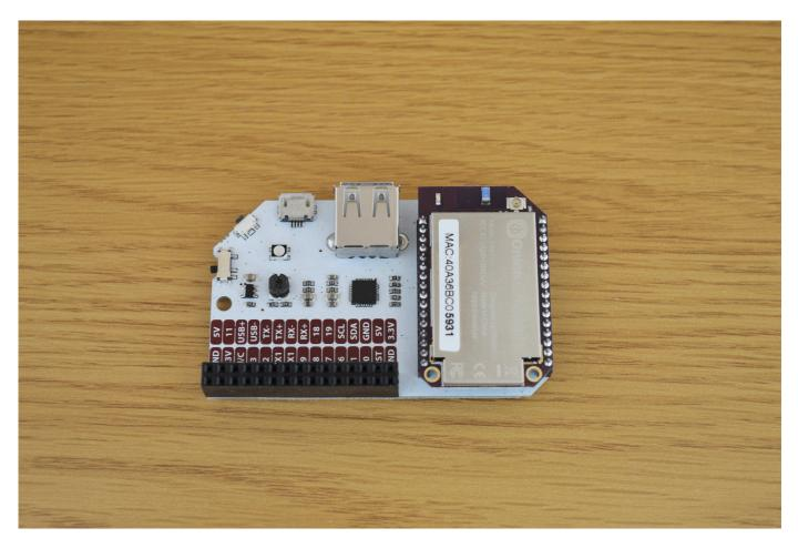
Make sure your Omega is pushed all the way down as demonstrated in the picture below:
