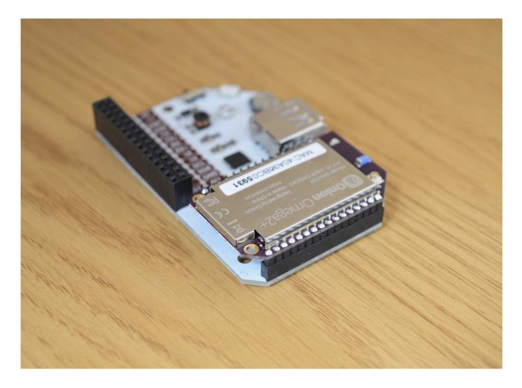
You may need to line up the pins with the holes before pressing the Omega into the Dock.
