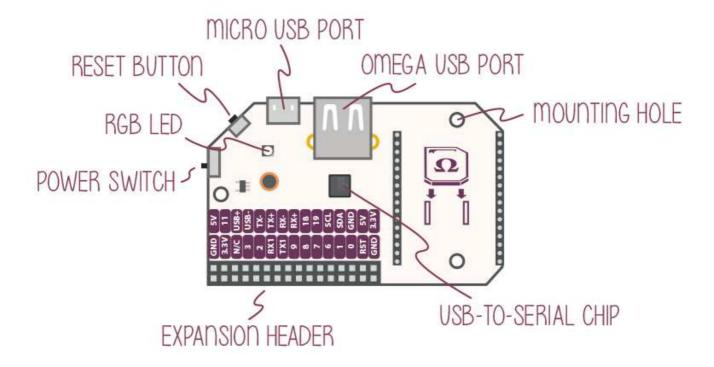
The Expansion Dock allows for easy communication via the USB-to-Serial chip located in the center of the board. You've also got a great RGB LED that you can control through the command-line interface.
