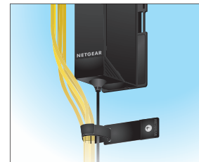
Strap the cables to the wall
