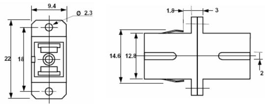
The SC has connector and adapter are the most used set for modern day optical fibre systems. With the audible click locking mechanism and pull proof design this connector provides a secure interconnect.
