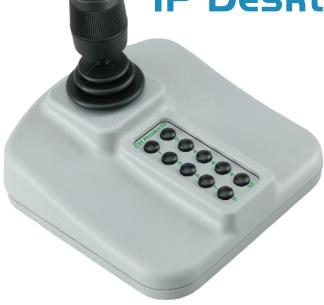
The IP Desktop USB joystick is designed to provide PC applications with responsive and accurate positioning controls. Featuring a three axis Hall effect joystick, twelve programmable switches and USB interface, the IP Desktop seamlessly integrates with software applications recognizing joystick inputs via Microsoft's DirectX.
