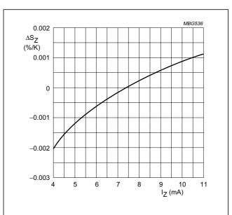
Fig.3 Temperature coefficient change as a function of working current; typical values.
