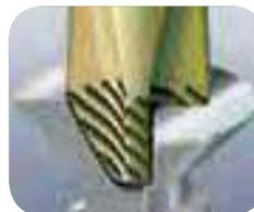
Screwdrivers can easily slip out of the screw, sometimes damaging expensive or important surfaces. The tip of Wera Lasertip screwdrivers has been microscopically roughened by a laser. This rough surface literally "bites" into the head of the screw. Accidental slipping becomes a thing of the past.
