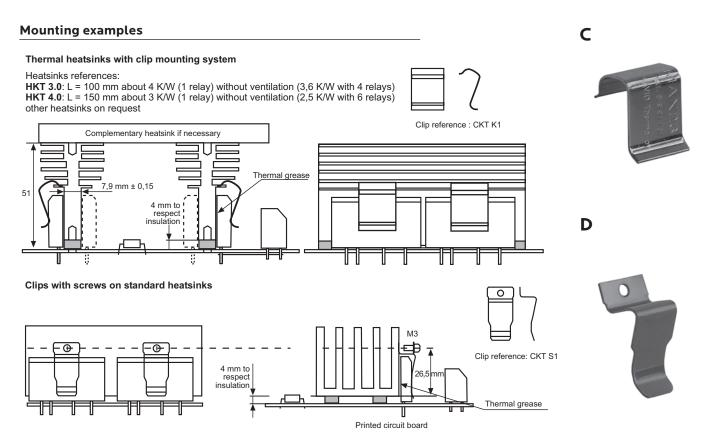
In each case, 4 mm must be respected between the printed circuit board and the heatsink, to keep a correct insulation between input and output (4 mm insulated washer). Mind to good contact between the relay and the heatsink. Use thermal grease.
