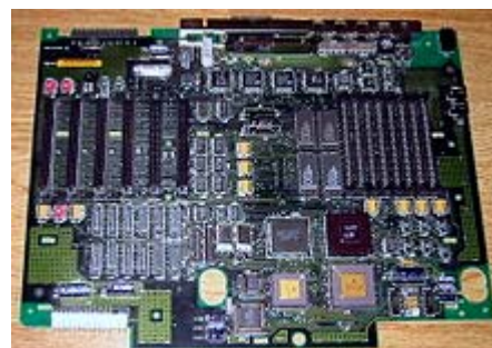
A NuBus motherboard, with six female 3x32 DIN 41612 connectors (black, centre left).
