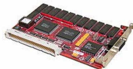
A NuBus graphics card with a male 3x32 DIN 41612 connector (white, foreground left).
