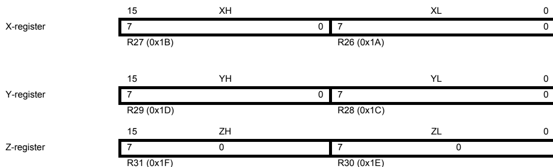
Figure 5-3. The X-, Y-, and Z-registers
