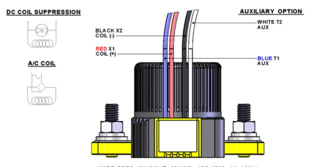
WIRE SPEC: SILICONE, 20AWG, -40C-150C, UL: VW-1
