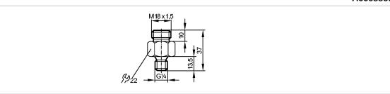
Made in Germany **Product characteristics** M18 x 1.5 - G 1/4 Adapter Insertion depth of the probe of SID, SFD, TN: 13.5 mm Environment 300 Pressure rating [bar] Mechanical data Housing materials stainless steel 316L / 1.4404 Weight 0.058 [kg] Accessories Accessories (included) sealing (AFM)
