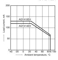
1-(2). Load current vs. ambient temperature characteristics
