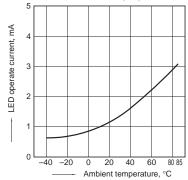
6. LED turn off current vs. ambient temperature characteristics Load voltage: Max.(DC); Continuous load current: Max.(DC)
