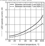
LED reverse current vs. ambient temperature characteristics
