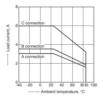
1.-(2) Load current vs. ambient temperature characteristics
