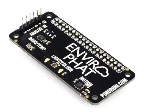
The Enviro pHAT packs 4 different sensors, letting you measure temperature, pressure, light level, colour, 3-axis motion, compass heading, and analogue inputs. It's ideal for monitoring conditions in your house or garage. Set up a web server with Flask and remotely monitor everything from anywhere. The board does require soldering for the header.
