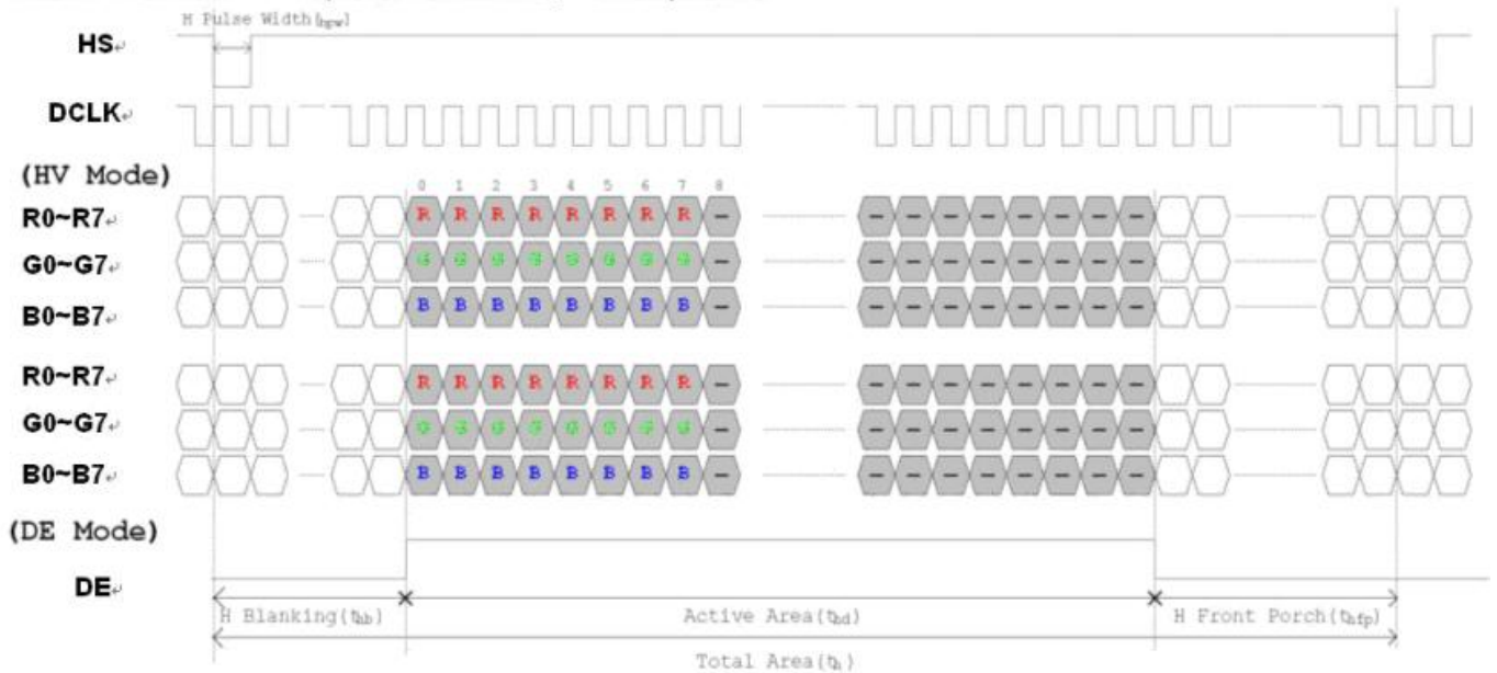
Horizontal input timing diagram.
