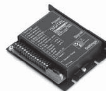
DEC 50/5 1-Q-EC Amplifier 1-quadrant amplifier for controlling EC motors with Hall sensors with a maximum output of 250 watts.
