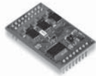
DEC Module 50/5 1-Q-EC Amplifier 1-quadrant amplifier for controlling EC motors with Hall sensors with a maximum output of 250 watts.
