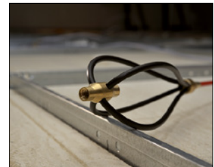
The whisk allows the rod to glide over obstructions easily.
