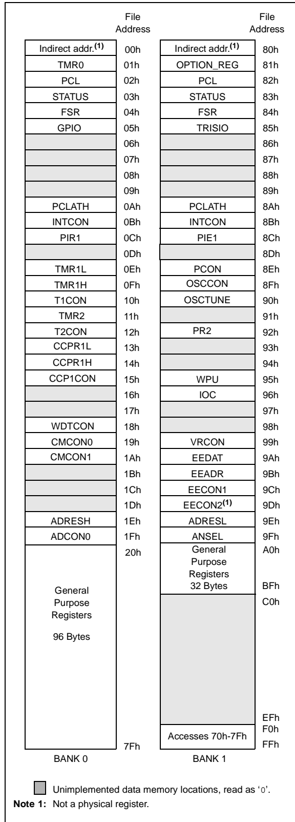
FIGURE 3-2: DATA MEMORY MAP OF THE PIC12F683
