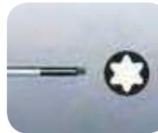
TORX® drive profiles transfer torque between tool and screw by line or surface contact rather than point contact as many other profiles. This protects both the screw and the tool profile. It also increases the amount of torque and power that can be transferred.
