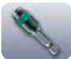
With the Wera Rapidaptor,  $\frac{1}{4}$ " bits can be inserted and automatically locked in the holder without using the slide switch. Even the smallest bits are easily removed by sliding the sleeve forward. The free-spinning outer sleeve stabilizes battery or mains-powered tools during the screwdriving process. All functions can be carried out with just one hand. There is no faster bit change!
