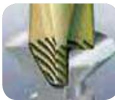
Screwdrivers can easily slip out of the screw, sometimes damaging expensive or important surfaces. The tip of Wera Lasertip screwdrivers has been microscopically roughened by a laser. This rough surface literally "bites" into the head of the screw. Accidental slipping becomes a thing of the past.
