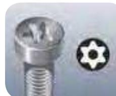
TORX® tools with a borehole prevent the unauthorised unfastening of safety screws. The screws contain a pin that protrudes into the drive profile so that "normal" TORX® tools cannot be used. This pin fits into the borehole of TORX® BO tools allowing safety screws to be unfastened.
