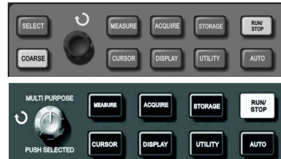
Figure 2-29 Function key (or cursor) of sampling system
