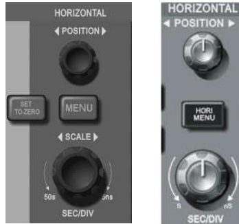
Figure 2-11 Interface of horizontal system
