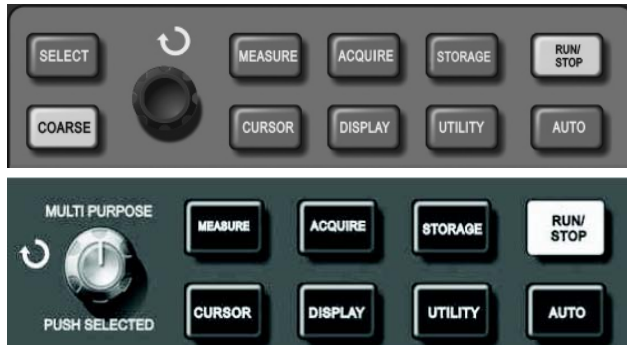
Figure 2–21 Function key of sampling system
