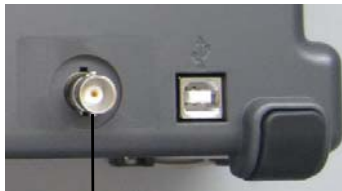
Rear panel of Pass / Fail output
