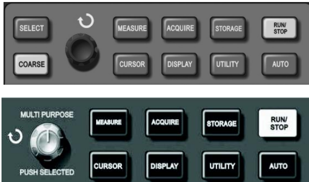
Figure 2—18 Function key of sampling system User can use ACQUIRE key to pop out sampling setup menu so as to adjust sampling mode by control button shown in the menu.
