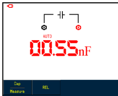
Figure 5-22 Measuring Capacitance in Relative Mode
