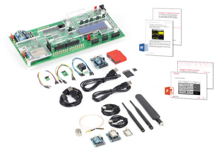
Figure 5: U3806A IoT Wireless Communications applied courseware, with training kit and teaching slides
