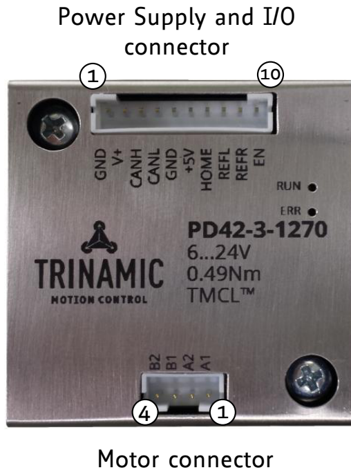
Figure 8: TMCM-1270 connectors
