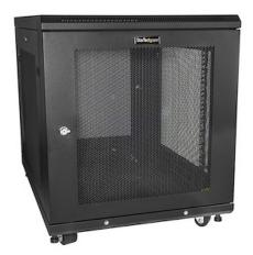
This server rack provides 12U of storage space in a sleek, secure cabinet for storing standard 19" rack-mount devices such as Dell, HP and IBM servers, along with telecommunication and A/V equipment. The rack is compatible with EIA-310 compliant equipment and supports a total load capacity of 450 kg (992 lb.).
