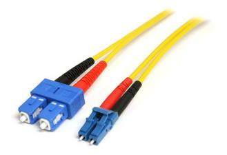
The SMFIBLCSC1 1m LC to SC Single-Mode Duplex Fiber Cable features 9/125 micron fiber for high-speed, high bandwidth data transmissions over Gigabit Ethernet and Fiber Channel networks, with support for duplex single-mode applications.
