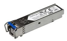
The SFPGE10KT3R5 is a Juniper SFP-GE10KT3R5 compatible fiber transceiver module that has been designed, programmed, and tested to work with Juniper brand switches and routers. It delivers dependable 1 GbE connectivity over fiber cable, for 1000Base-BX10-U compliant networks, with a maximum distance of up to 10 km (6.2 mi).
