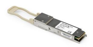
The QSFP40GSR4ES is a Dell EMC QSFP-40G-SR4 compatible fiber transceiver module that has been designed, programmed and tested to work with Dell EMC brand switches and routers. It delivers dependable 40 GbE connectivity over fiber cable, for 40GBase-SR4 compliant networks, with a maximum distance of up to 150 m (492 ft).
